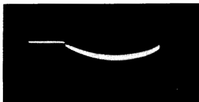
Fig. 1015 (left). Time-base-triggered spurious oscillation in the Y amplifier. Fig. 1016 (right). Spurious oscillation in the Y amplifier triggered by the time-base return stroke.
