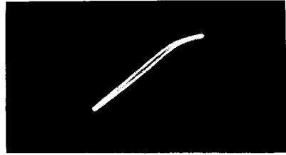
Fig. 708 (left). Insufficient bias rounds the tops of the waveform. Fig. 709 (right). Characteristic corresponding to the condition shown in Fig. 708.
