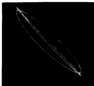
Fig. 639. Phasing ellipses obtained with the circuit of Fig. 638.
