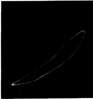
Fig. 617 (left). Looped characteristic due to phase shift. Fig. 618 (right). Circuit used for producing the I_p/E_g characteristics of triodes.
