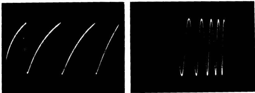
Fig. 226 (left). Reducing the bias results in a less curved sawtooth wave. Fig. 227 (right). Sweep obtained with the sawtooth wave of Fig. 226. The crowding of the trace is much less marked.
