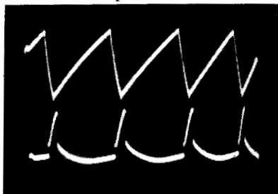
Fig. 242. Same as Fig. 241, but time constant of R1C1 in Fig. 240 is different.
