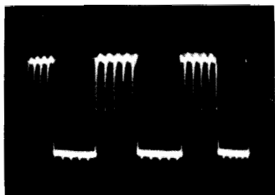
Fig. 550 (left). Waveform produced by mixing a 500-cycle square wave and 5,000-cycle pulses. Fig 551 (right). Waveform produced by mixing pulses of 500 and 5,000 cycles.
